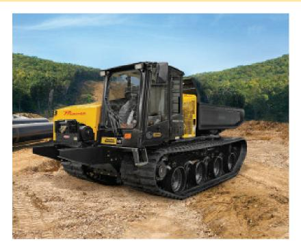
PipeLine Machinery International (PLM) presents the latest custom equipment solution – the PANTHER T12 by PRINOTH. Just like it's predecessor, the T8, the T12 is the latest innovation in a low ground pressure crawler and operates in off-road and various weather conditions offering exceptional performance and versatility in mining, construction, oil and gas (pipeline) as well as electric utility sectors.
