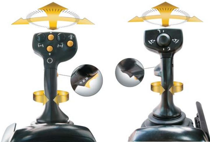
Operators are more comfortable and productive with two electro-hydraulic joysticks. Electronically adjustable control pods help position operators for optimal visibility and proper operation.
