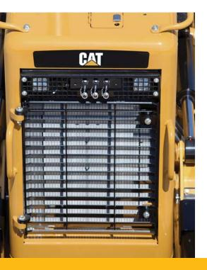
The radiator, air-to-air aftercooler and hydraulic oil cooler are packaged in a single plane, making cleanout easier. Durable, aluminum bar plate construction gives you superior heat transfer and corrosion resistance. 8.9 fins per inch (6.5 fpi on Waste Handlers) on the standard core allow debris to pass through and help reduce plugging.
