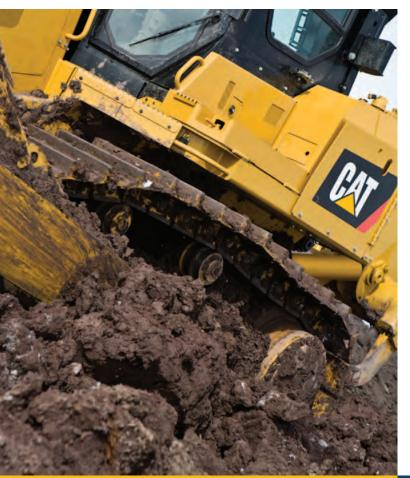
The D7E features an advanced low drive undercarriage design for greater machine versatility in a wider range of applications. Enhanced visibility, especially to the sides, is only one of the many benefits of this highly efficient undercarriage system.
