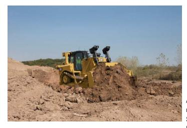
A Cat C15 ACERT engine gives you the power and reliability you need to get the job done. Improved fuel economy over Tier 4 Interim/ Stage IIIB/Japan 2011 (Tier 4 Interim) and efficient use of Diesel Exhaust Fluid (DEF) gives you excellent overall fluid efficiency.
