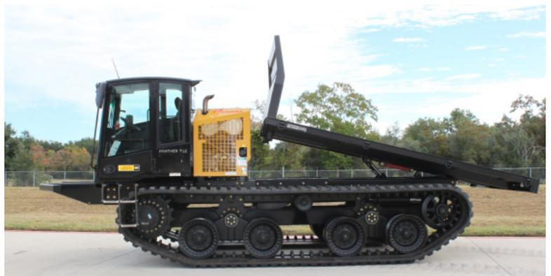
Built with a truck-inspired widened chassis to accept virtually all implements without any modifications, the PANTHER T12 is pictured here with a tilting flat bed. From construction to right-of-way maintenance, in the middle of nowhere or within city limits, both the PANTHER T8 and the T12 have the toughness, tenacity and reliability you need in a crawler.
