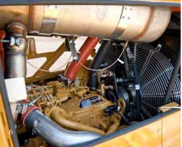
Emissions reduction technology on the D6N is designed to be transparent, with no action required from the operator. Low temperature regeneration runs automatically in the background while you work.
