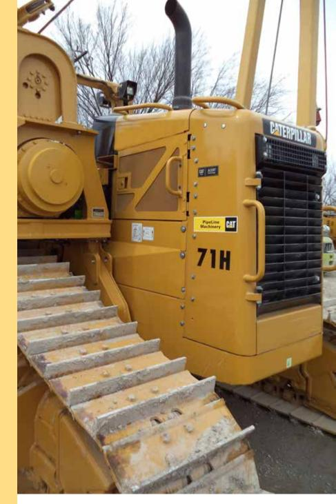
Pipeline Machinery International (PLM) has developed a pipelaying solution to enhance its pipelayer offerings. With the support of Caterpillar and the engineering expertise of Vanguard Equipment Inc., the challenge was met to create a utility-capacity pipelayer in the Tier 4 Final / Stage IV emissions class, designed for lifting 27 215 kg (60,000 lb.) and engineered to meet the most exacting standards in the world.
