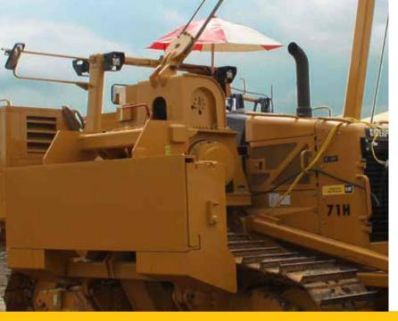
The 71H main frame is engineered to handle the unique demands of the pipelaying operation.
