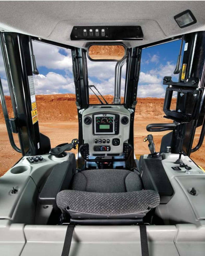
An isolation-mounted pressurized cab reduces dust, noise and vibration. Large glass panels provide excellent visibility. Intermittent wipers maximize visibility in poor weather conditions. Cab (ROPS) mounted air conditioning gives you more cooling capability, and removes the condenser from under the hood so it is easier to service.
