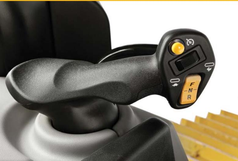
All controls are electro-hydraulic, which means precision and maneuverability. They are ergonomically designed for easy intuitive, comfortable and low effort operation. Blade response can be adjusted through the operator profile in the display.
